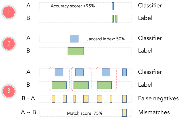
Figure 14: Enhanced performance analysis through visual track algebra. Track Xplorer lets data scientists reason about the tradeoffs of each performance metric, helping them decide which ones to adopt. It also helps them gain insights for developing new, effective performance metrics tailored to the classification task at hand.
