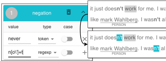
Figure 5: Left: Example concept created to capture negation. Right: example text highlighting as concept elements are matched in the text, and annotations created once the element is submitted.
